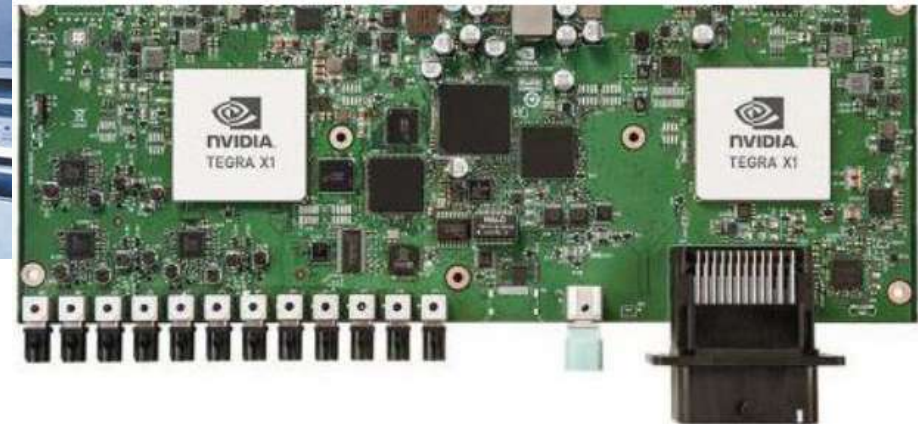
The nVidia PX computing system for autonomous vehicles (2015).
