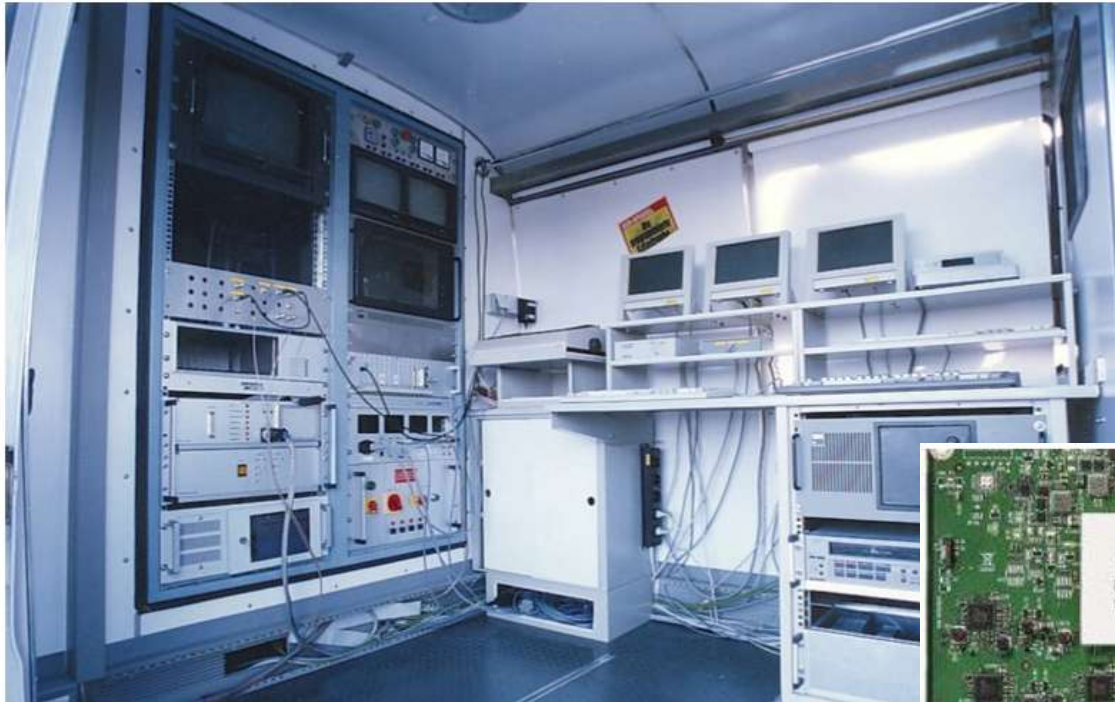
The computing system used in Ernst Dickmann's VaMoRs van (1987).
